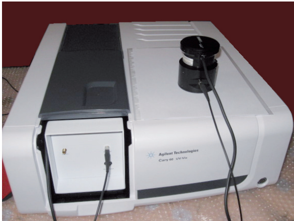
Figure 1: Agilent Cary 60 UV-VIS with the remote fiber optic diffuse reflectance accessory (DRA).
